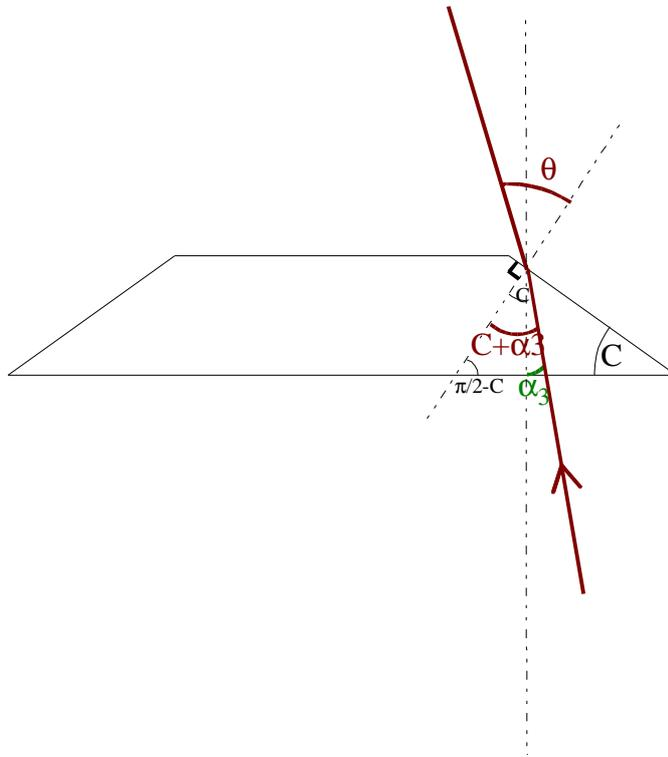
On a :  $\sin \theta = n \times \sin (C+\alpha_3)$  , soit:  $\sin \theta = n \times \sin \{C + 4P + i -180^\circ\}$
